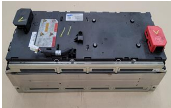
Fig. 1 Image of electric bus used battery module
