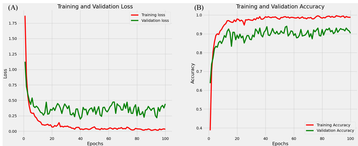
Fig. 3. Training and validation loss (A) and accuracy (B) of the DenseNet201 model. The hyperparameters used to perform training were 9 classes, 20 epochs, a batch size of 128, Adam optimizer, and a learning rate of 0.001.
